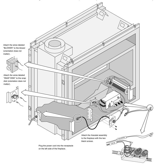
Attach the brown and red wires to the front of the gas control valve as shown above (wire color orientation does not matter). The blue wires are for the optional modulating remote (do not connect at this time).
